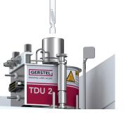
Stir Bar Sorptive Extraction (SBSE), based on the GERSTEL Twister<sup>®</sup>, is a solvent free technique for ultratrace determination of organic compounds in aqueous matrices. The PDMS or EG-Silicone phase on the Twister efficiently extracts organic compounds while the sample is stirred. SBSE is up to 1000 times more sensitive than
