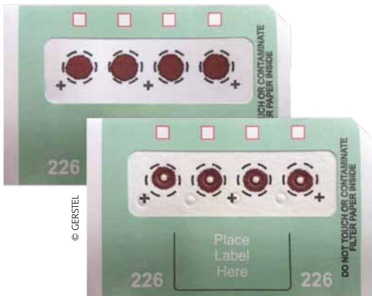
DBS desorption is performed with high accuracy in the user-defined section of the blood spot. Quantitative recovery is achieved resulting in high reproducibility.
