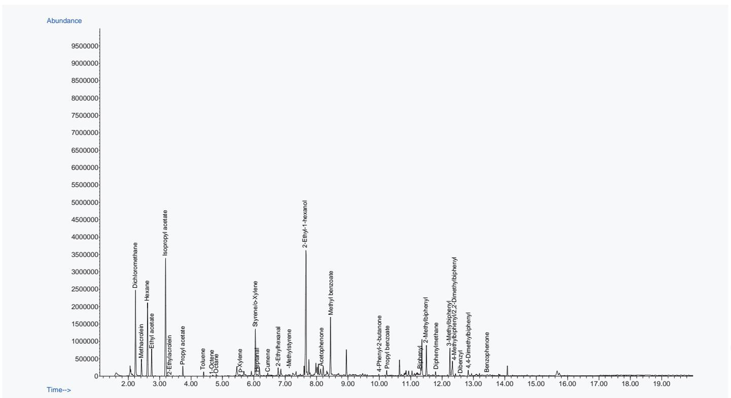
Figure 6: Total ion chromatogram for floor tile sample.
