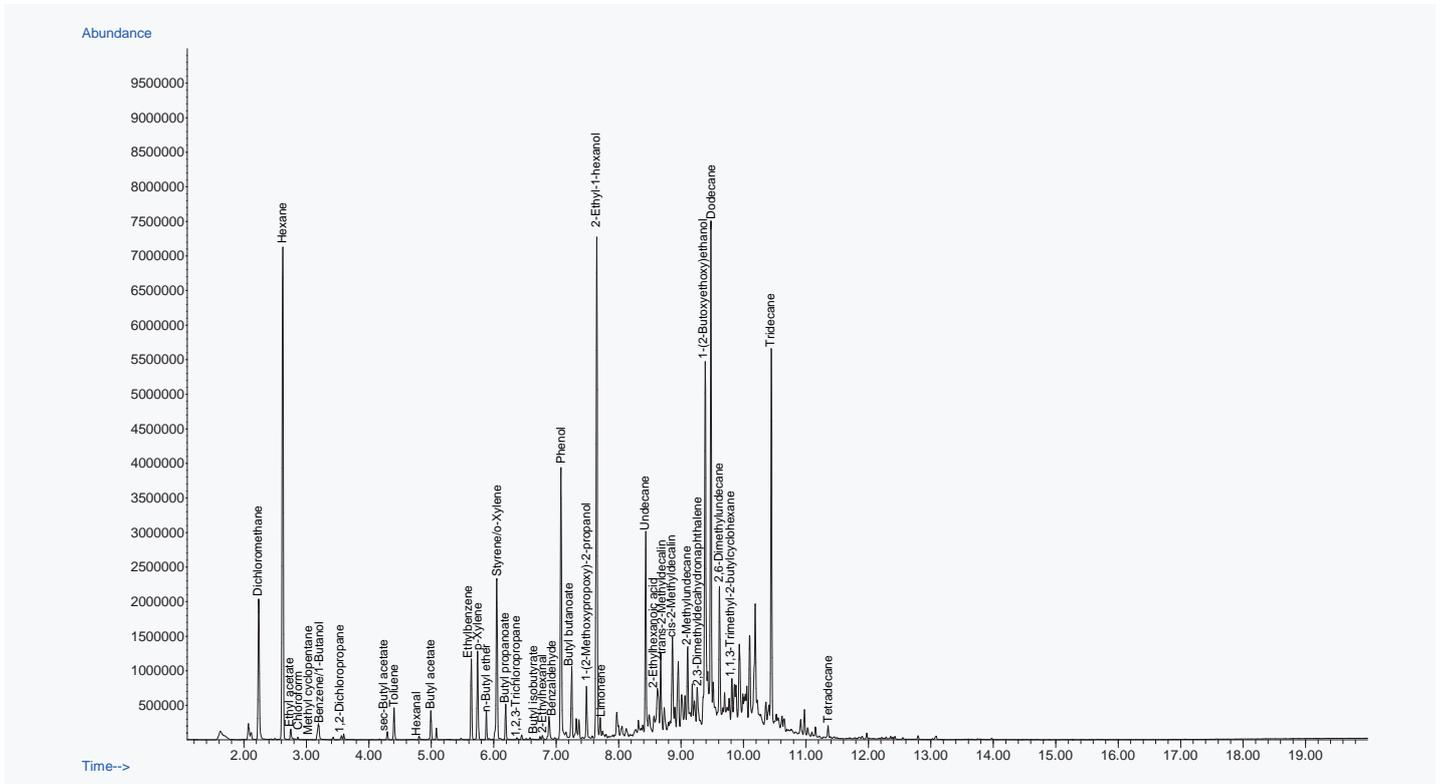
Figure 5: Total ion chromatogram for wallpaper sample.
