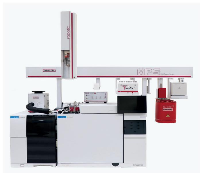
**Figure 2:** DHS L system coupled with TD-GC/MS.
