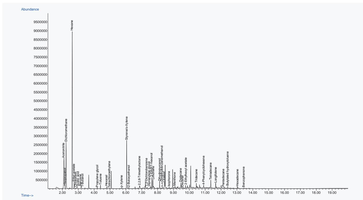
Figure 4: Total ion chromatogram for carpet sample.
